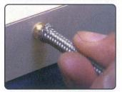
Step Two: Insert the nipple portion of the PowerFlex hose end in a vise. Slip the hose over the nipple using a twisting motion to size the I.D. of the teflon. Separate the wire braid from the O.D. of the Teflon® tube with a small screwdriver. Be careful not to crush the Teflon.
