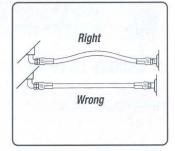
Allow slack in your hose assembly for changes in length that occur under pressure.
