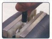
Step Two: Unscrew socket from hose end. Push hose into socket, turning counter-clockwise, until hose is seated against step in socket. Make sure rubber part of hose does not protrude into socket threads.
