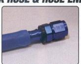
Step Two: Liberally oil inside of hose & barbed end of hose end. Insert barbed end into hose using a twisting action. Put the swivel end at center hex in a vise. Use a twisting motion make bottom of hex even with nose edge, rubber insulator will cover end of hose.
