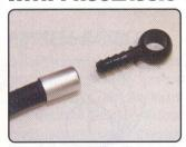
Step Three: Apply Russell Assembly Lube (or oil) onto barb assembly. Start barb assembly into hose; grasp hose behind collar & push hose onto barb assembly until it has fully bottomed out at collars edge.
