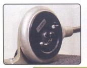
Step Five: Make sure your die number is correct for hose you are crimping. Lift handle to top position opening dies. Place end assemble in dies. Align edge of the collar (at hose) with back face of dies, using over center action push down on handle until assembly releases from crimper. Inspect assembly, be sure to wash & pressure test prior to use.
