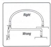
When routing the hose assembly, provide a smooth bend radius. Avoid sharp bends, which will collapse the hose I.D. and could restrict flow.
