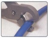
Step One: Cut hose to length using a sharp knife or shears.
