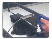
Step One: Wrap the hose tightly with electrical or racers tape. Hold the hose firmly in a vise without crushing and cut through the tape. Make sure you make a straight cut. Remove the tape slowly and deburr the Teflon® edges. Install the socket on the hose and slide it back out of the way.
