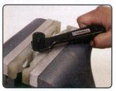
Step Four: Hold socket/hose in vise. Turn nipple with wrench until there is less than 1/16" between nipple hex and socket. Repeat Steps 1-3 for other end of hose. Then, flush hose assembly with solvent or soapy water and blow clean with compressed air or let air dry.
