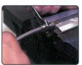
Step Four: Start the socket onto the nipple by hand. Tighten with a wrench until the gap between the nipple and the socket is no more than 1/16". Clean the hose assembly and pressure test before using.
