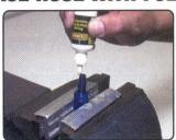
Step Three: Position the nipple assembly of the hose end in the vise using soft jaws. Apply assembly lube to the threads of the socket as well as to the nipple assembly.
