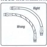
Avoid installing the hose in a twisted position.
