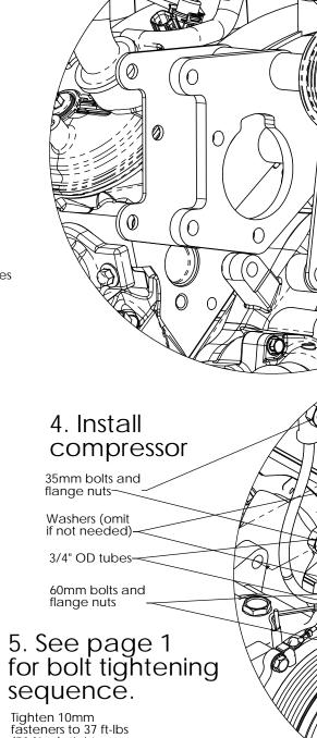
(50 N-m), tighten 12mm fasteners to 50 ft-lbs (68 N-m) Performance, Inc. www.kwikperf.com
