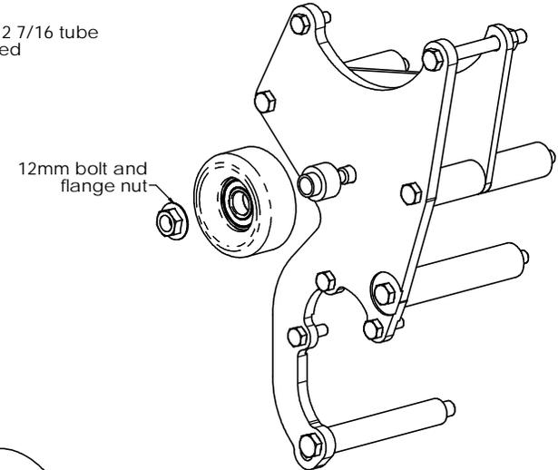
4. Attach alternator. Tighten 8mm bolt to 15 ft-lbs. Tighten other fasteners to 25 ft-lbs.
