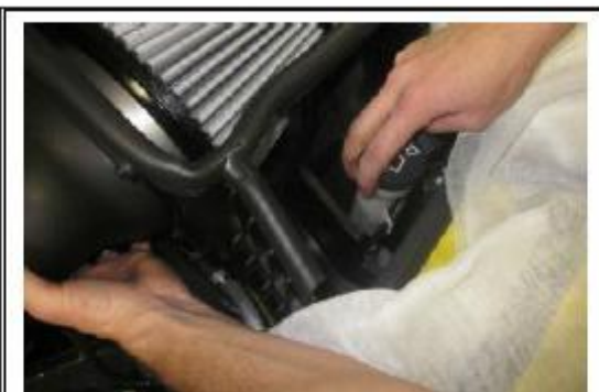
Figure 2: GENTLY move parts as needed to lower airbox in place
