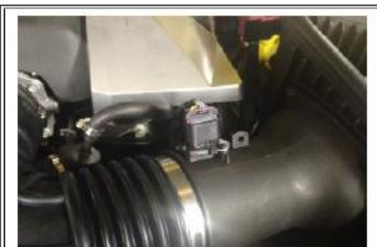
Figure 3: Reinstall MAFS wiring and retainer
