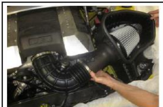
Figure 1: Maneuver intake system into vehicle position
