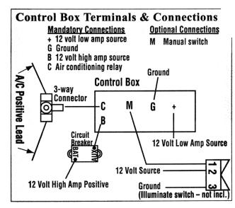
IMPORTANT: If not using an illuminated switch, disconnect the switch ground.
