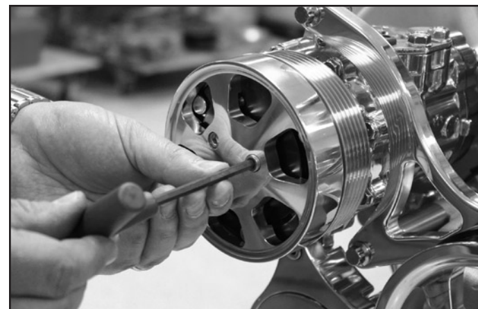
Figure 13: Install Compressor Clutch Cover
