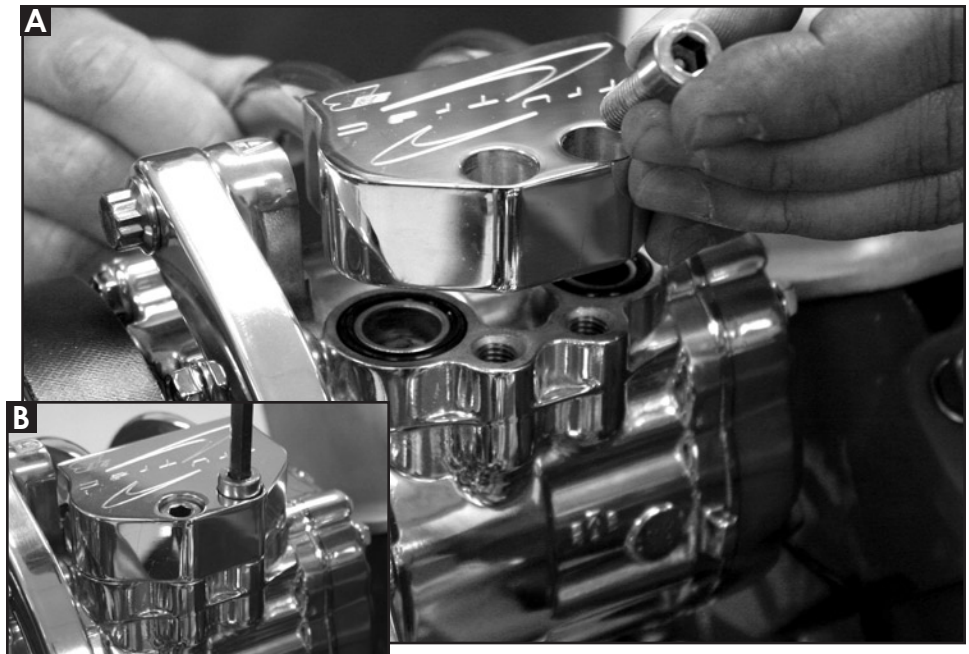
Figure 15: Install Compressor Manifold
