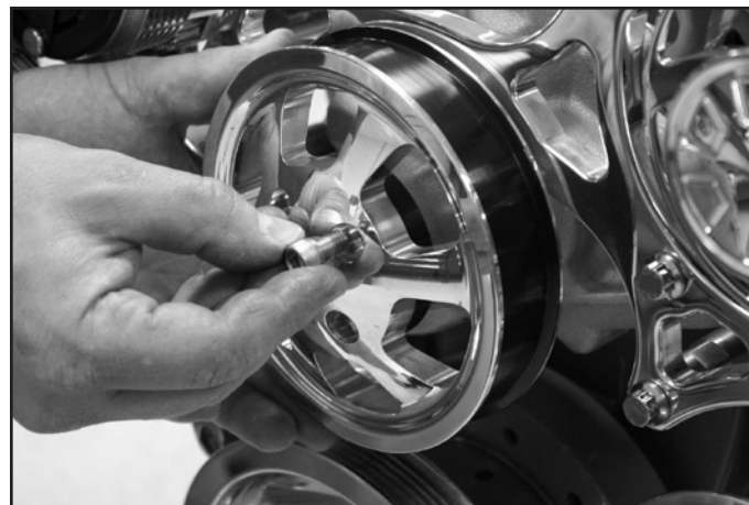
Figure 12: Install Water Pump Pulley
