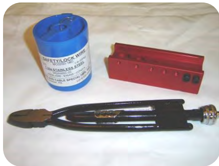
Shown is Drill bolt fixture, stainless wire & safety wire pliers.
