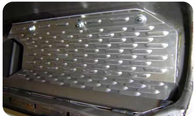
Photo of the louvered windage tray.
