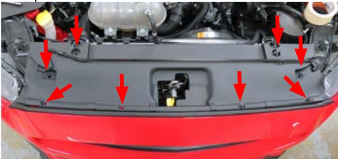
4. Remove six (6) bolts securing the top of the fascia using an 8mm socket.
