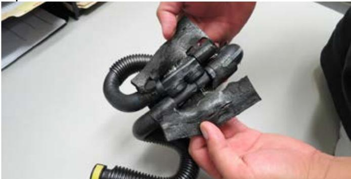
77. Remove the hose that attaches to the check valve and replace with the supplied 3/8" hose. Attach the supplied vacuum cap to the opposite end of the aspirator.
