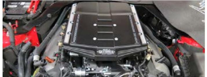
65. Mount the fuel rails and move them away from the supercharger to access the supercharger manifold bolts. Secure the supercharger manifold to the cylinder heads using a 10mm swivel socket to install ten (10) M6 x 30mm intake manifold bolts supplied in hardware Bag # 1. Using the torque sequence below, torque the bolts to 8 ft-lbs.
