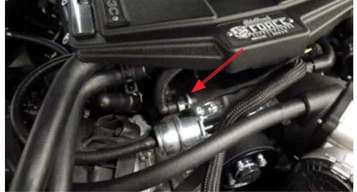
72. Remove the evap solenoid from the factory manifold. Install the solenoid onto the bracket using the factory rubber grommet. Connect the hoses. Put the evap in position and leave the bracket loose until the supercharger installation is complete.
