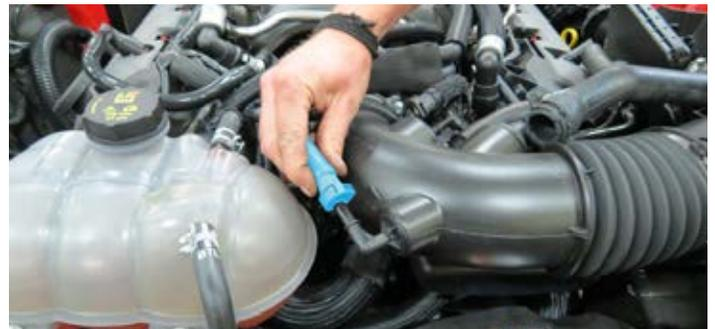
20. Disconnect the brake aspirator hose from the manifold PCV hose.
