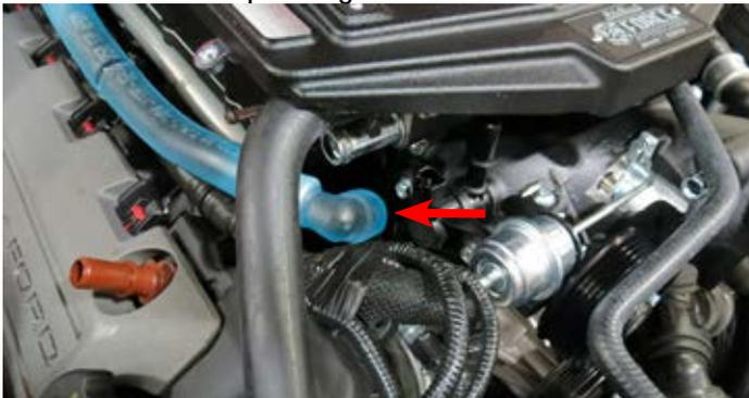
71. Install the supplied evap hose with 90 degree fitting onto the nose,
