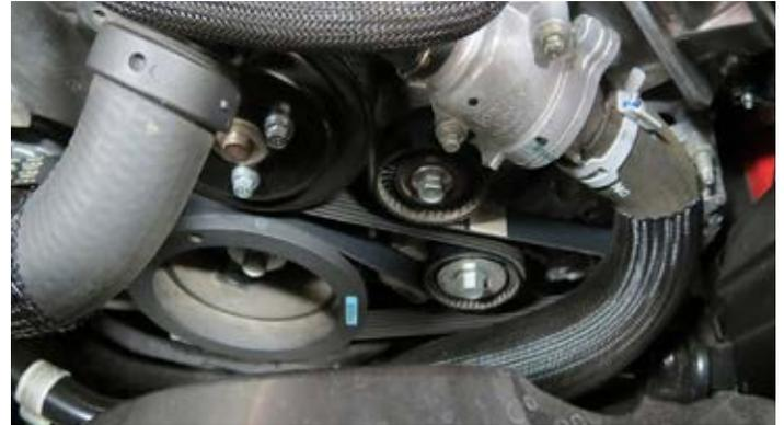
42. Remove the two (2) indicated engine cover bolts using a 10mm socket. Using a 90° drill and the supplied drill bit, drill out the indicated hole on the front engine cover 1.01" deep. **(NOTE: The center hole on some vehicles will already be drilled and tapped by the factory. Please inspect your front cover and avoid drilling this hole if already tapped.)** If not already tapped, the hole in the center should be drilled .72" deep. All holes should be tapped to M8 x 1.25 with the supplied tap.
