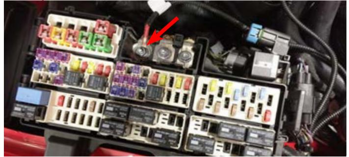
101. Route the "Intercooler Water Pump" end of the Water Pump/EVAP Harness below the fuse box and around the washer fluid reservoir and plug it into the intercooler water pump.
