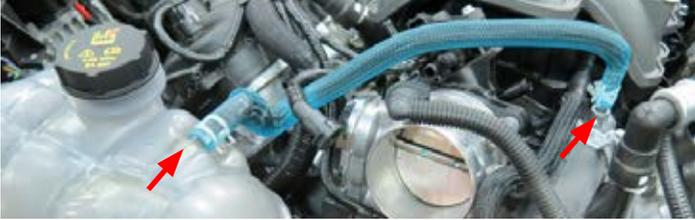
54. Remove the O-ring manifold gaskets from the factory manifold and install them onto the supercharger runners. Apply a small amount of O-ring lubricant to the exposed area of the gaskets. This will help prevent tears during installation of the supercharger.
