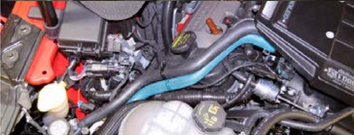
93. Attach the surge tank bracket to the surge tank using two (2) M6 x 10mm bolts from Hardware Bag # 3. Also attach the water pump hose to the surge tank and secure it with a hose clamp from Bag #3.
