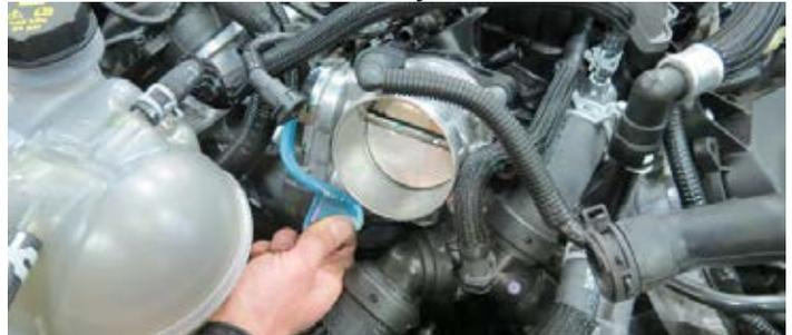
28. Using an 10mm socket, remove four (4) bolts securing the heater hose retaining brackets.
