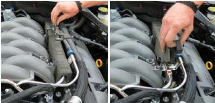
30. Disconnect eight (8) fuel injector connectors.
