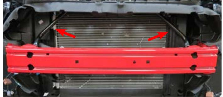
85. Back out the four (4) crash beam bolts (circled in image) but do not remove. Install the LTR brackets from behind the crash beam and onto the crash beam support studs. Line up the holes on the LTR brackets with the studs to temporarily hold the LTR brackets in place. Then install the LTR from below as pictured.
