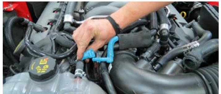
21. Using a flathead screwdriver, loosen two (2) worm clamps securing the air inlet tube and remove.
