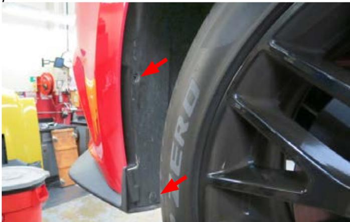
8. There is an additional push pin located just above the tire that needs to be removed.
