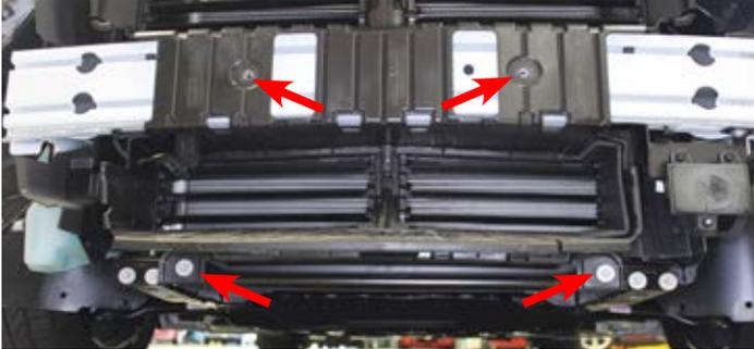
82. Remove the two (2) clips securing the shutter bracket to the core support.
