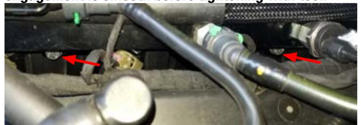
67. Reconnect the injector connectors to the appropriate fuel injectors. **WARNING: Never attempt to rotate the injectors.**
