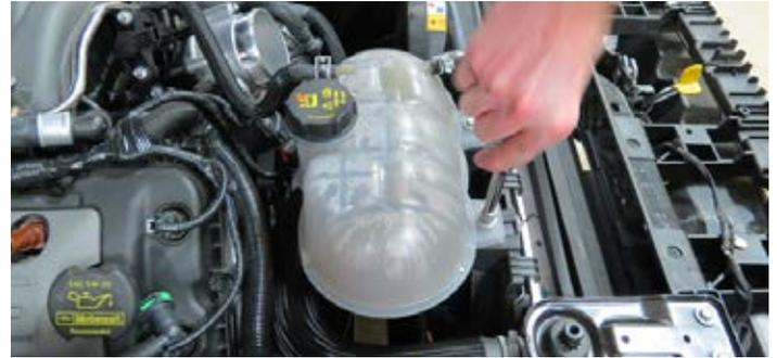
40. Position the coolant reservoir tank out of the way to access the drive belt tensioner.
