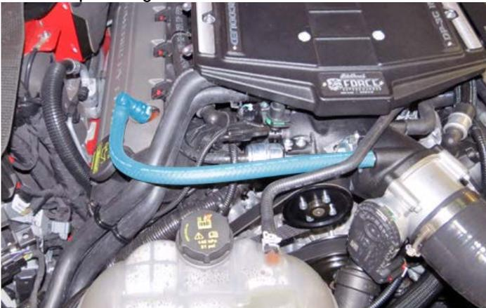
99. Zip tie the Fuse holder on the Water Pump/EVAP Harness onto the fuse box.
