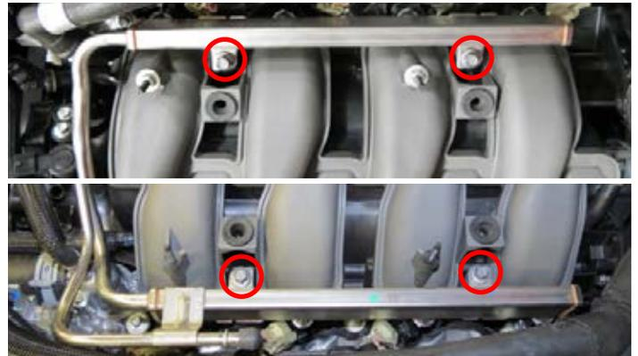
34. Using an 8mm socket, remove six (6) manifold bolts.
