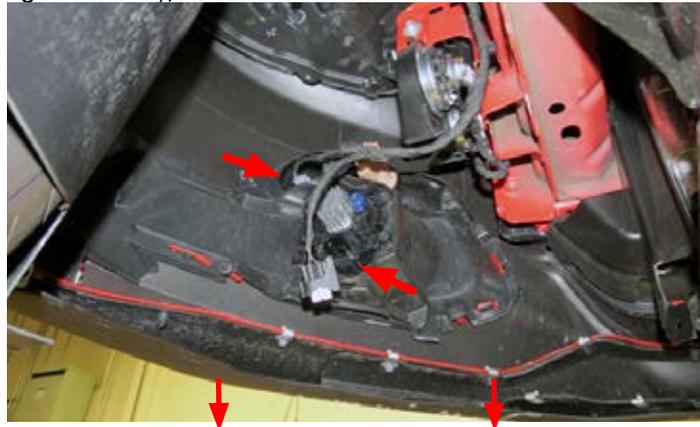
12. Tape up the fender as needed to prevent scratching the painted surfaces. With the help from an assistant, carefully disengage both sides of the fascia by gently pulling the sides outwards. Remove the fascia and set aside.
