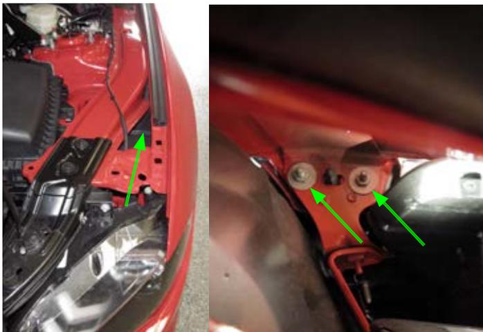
10. From within the wheel well remove the fascia retention assembly that the nuts were removed from in the previous step. Pull downward until the plastic pin no longer retains the assembly. Remove from vehicle, ensuring to distinguish between passenger and driver side.
