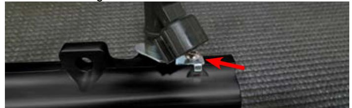
60. Remove the factory fuel pressure sensor from the driver side factory fuel rail.
