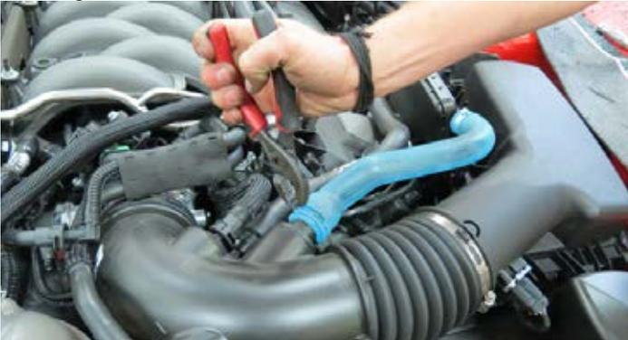
17. Remove the brake aspirator hose from the air inlet tube.
