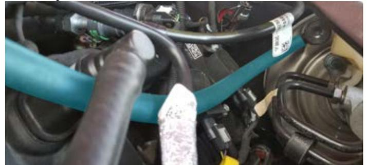
80. Route the Aspirator to Manifold hose under the heater hose and attach to the fitting on the supercharger nose.
