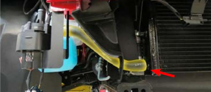
92. Insert the LTR to Manifold hose through the hole on the upper shroud and secure to the top LTR bung with a hose clamp from Bag # 3. Secure the other end to the lower bung on the supercharger manifold.
