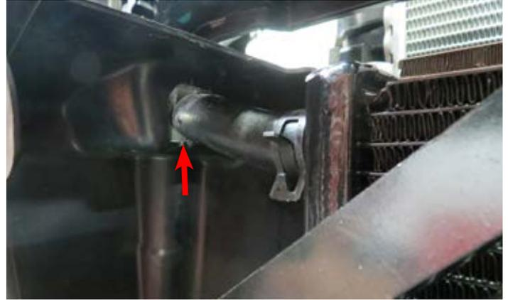
89. Attach the LTR to WP hose to the water pump and secure with a hose clamp from Bag # 3.
