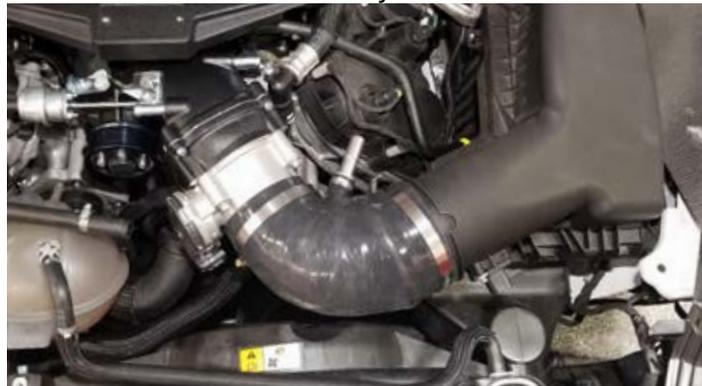
108. Connect the brake aspirator to the lower fitting on the silicone elbow.
