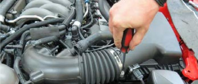
22. Disconnect the EVAP connectors and fully remove the EVAP hose .
