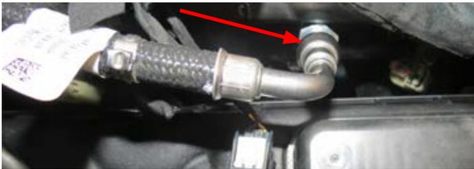
69. Reinstall the passenger side heater hose fitting using the factory hardware.
