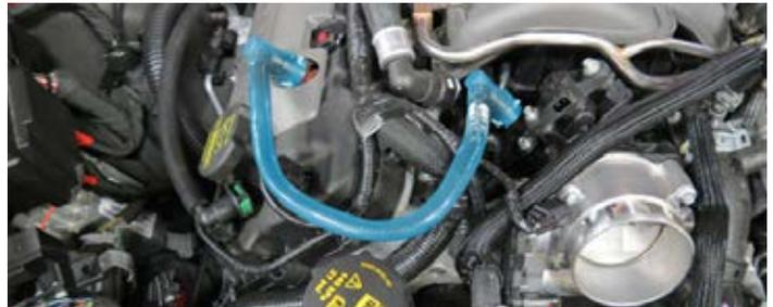
27. Disconnect the throttle body connector.
