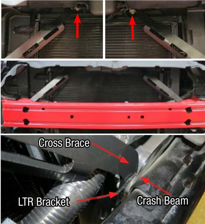
87. Using a drill and a 1 1/4" hole saw bit, drill a hole in the shroud that lines up vertically and parallel with the lower LTR barb.
