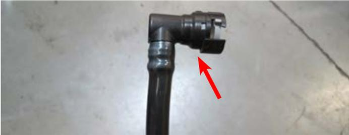
98. Attach the 90° fitting onto the supplied 1/2" Cadbar hose. Connect the quick connect fitting to the passenger side valve cover and the other end of the hose to the barb on the supercharger nose.
