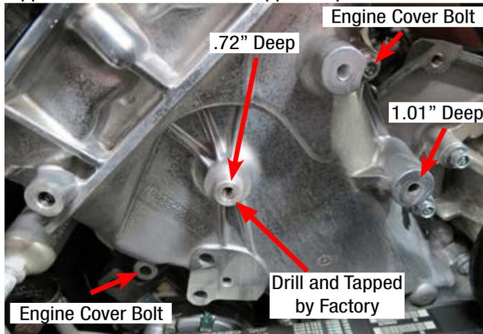
43. Secure the new tensioner bracket to the bosses that were just drilled and tapped with bolts supplied in Bag # 2.
