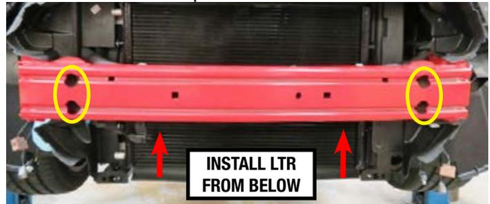
86. Install the supplied cross braces using the two (2) M8 x 30mm hex flange bolts from Bag # 3, loosely screw in the bolts through the crash beam braces. The lower cross braces will sandwich the LTR to the crash beam and be secured using the M8 nuts and washers supplied in Bag # 3. Once all bolts are in place through the braces, fully tighten the bolts and nuts.
