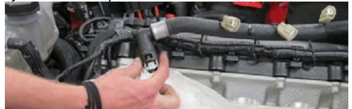
52. Remove the passenger side heater hose fitting with an 8mm socket. Repeat for the driver side heater hose fitting. Temporarily plug the holes with a rag.
