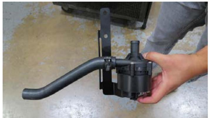
90. Feed the hose through the hole in the shroud and secure the water pump to the chassis using the supplied nuts in Bag # 3.
