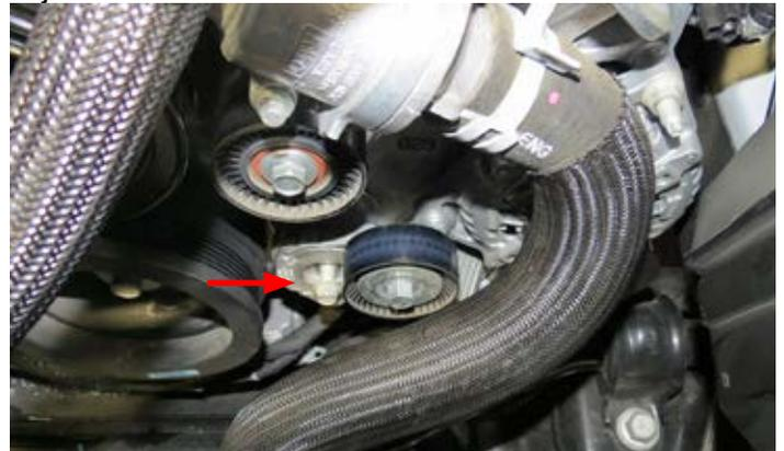
45. Remove both the engine cover bolt using a 10mm socket and the bolt through the ear of the alternator using a 15mm socket.
