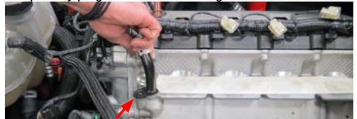
53. Using a hose clamp tool, remove the factory coolant bleed hose from the reservoir and bleeder fitting.
