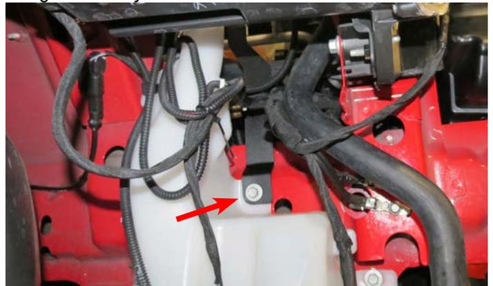
97. Using a razor blade, or equivalent, remove the 90° quick connect fitting on the factory passenger side PCV hose.
