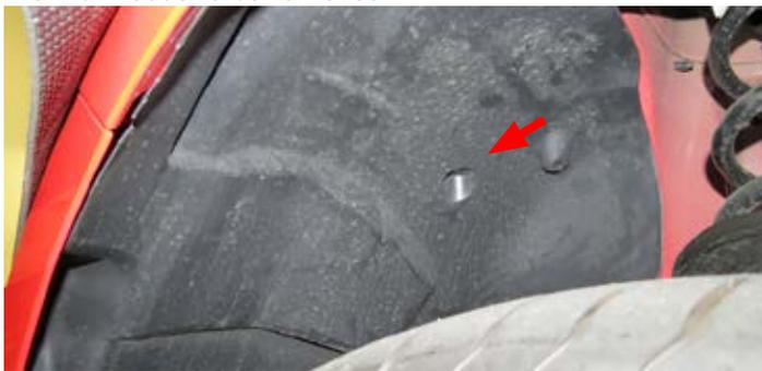
9. Reaching through the shown opening, remove four (4) nuts, two per side, securing the fascia to the fender using a 10mm socket.
