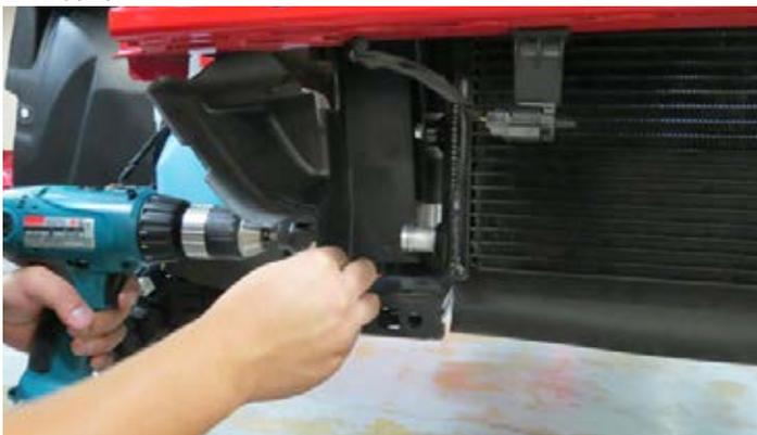
88. Cut a hole in the shroud that the upper LTR hose can route through. **CAUTION:** Be mindful of the A/C hard lines behind the shroud.
