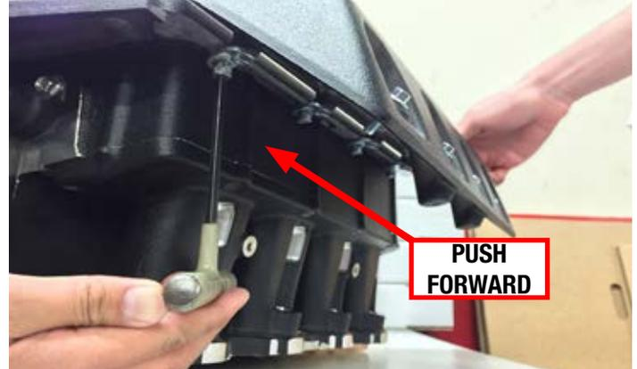
57. Using O-ring lube, install the fuel caps onto the fuel rails. Attach the supplied fuel crossover to the rear of both rails. Insert the straight fittings into the fuel rails as shown.
