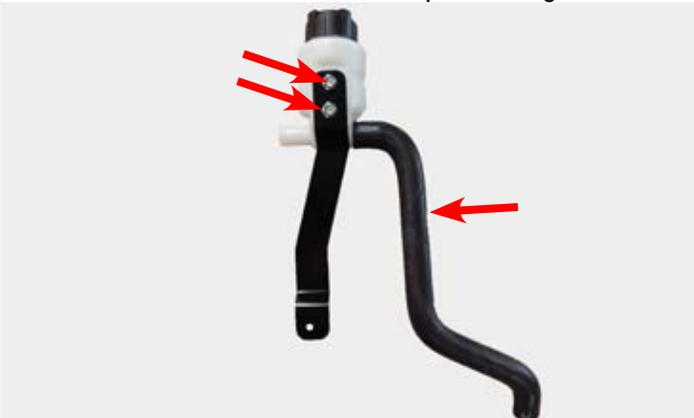
94. Connect the Water pump to Surge tank hose to the water pump and secure with a hose clamp from Bag #3.
