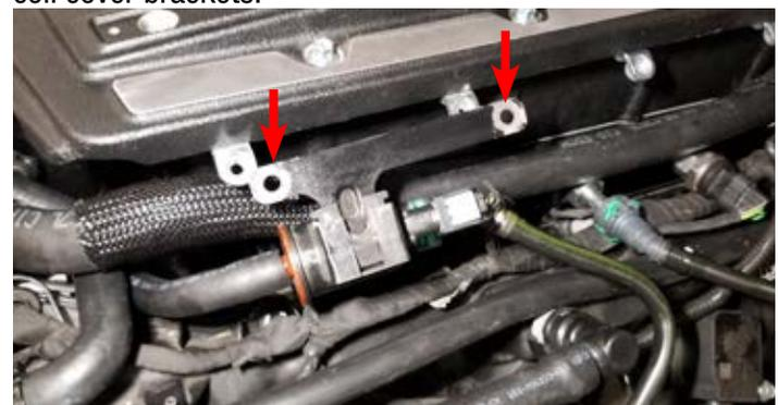
134. As a precaution, slice a 5" length of hose to wrap around the fuel line as pictured. This is to prevent the hose from rubbing on the edge of the coil cover. Secure with zip-ties.
