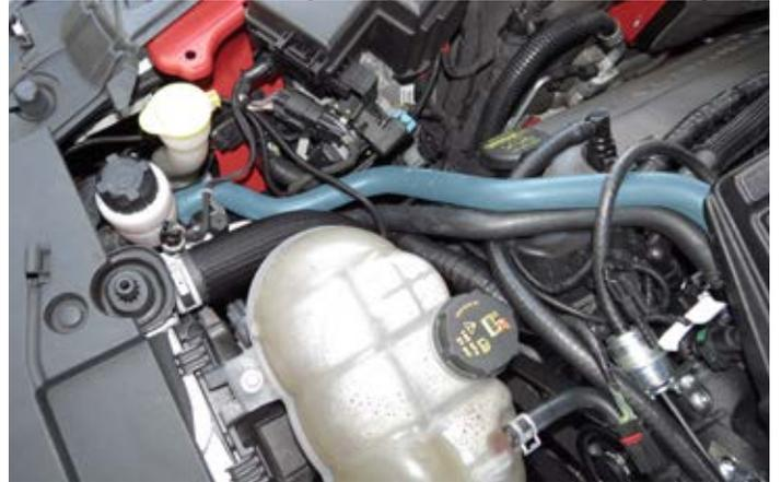
96. Using a 10mm socket, remove the top bolt securing the windshield wiper fluid reservoir. Place the surge tank bracket onto reservoir and secure the bracket and reservoir using the factory bolt.
