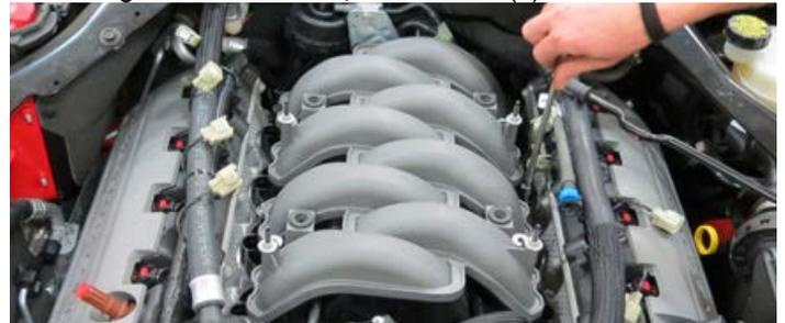
35. With the stock manifold remaining in the vehicle, rotate and manipulate it until you are able to remove the 4 connectors from the rear of the manifold as shown below. Disconnect any plastic anchors from the back of the manifold.
