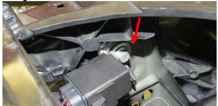
103. Route the ground strap and water pump connector downward through the frame. Remove the bolt securing the factory ground shown and mount the ground strap along with the factory ground in the original location. Connect the water pump.
