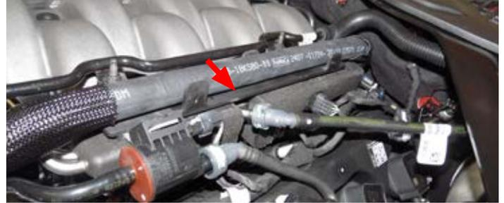
32. Repeating spill protection procedures from step 46, remove the fuel line from the passenger side fuel rail. Use a 3/8" fuel line disconnect tool to remove the line.
