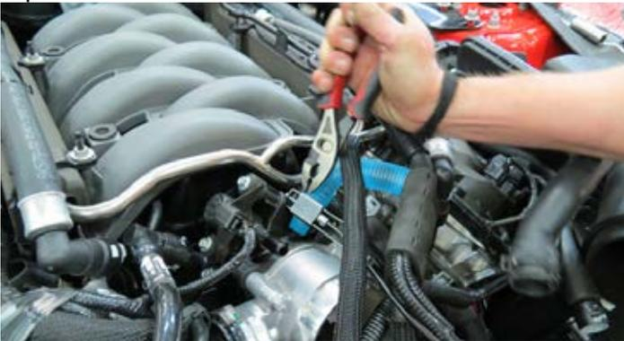
24. Remove the brake aspirator hose assembly from the brake booster and set aside as it will be reused later.
