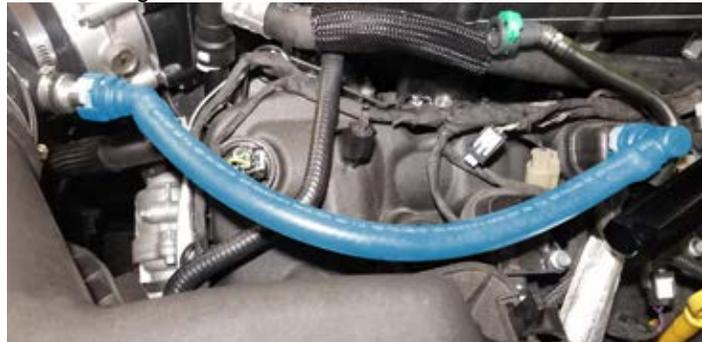
110. Separate the MAF harness connector from the MAF sensor located at the outlet of the airbox. Connect the engine harness to the connector on the MAF/Temp harness then attach the MAF/Temp harness to the MAF Sensor. Reattach the harness to the tab on the airbox.
