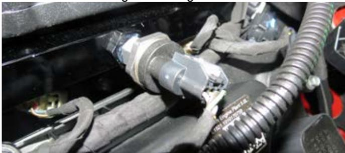
62. Temporarily install the fuel rail assembly onto the supercharger manifold.
