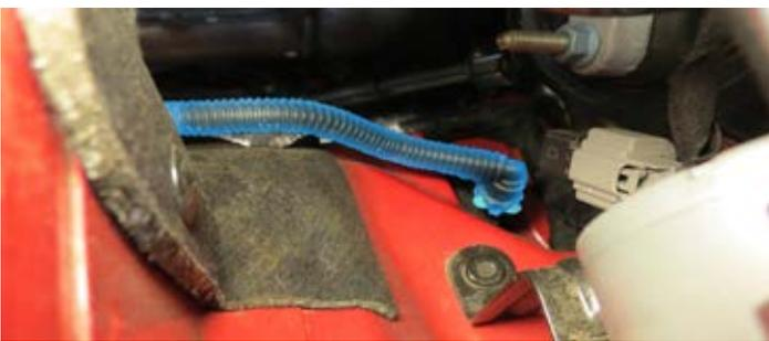
23. Using a hose clamp tool and pliers, remove the brake aspirator hose from the intake manifold.
