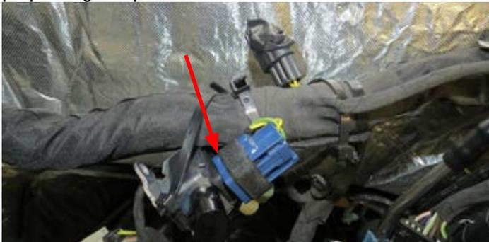
38. Tape up the end of the two (2) IMRC position sensor plugs and secure plugs to the main harness out of the way. These will not be reused.
