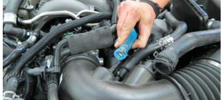
18. Remove the driver side PCV hose from the air inlet tube.
