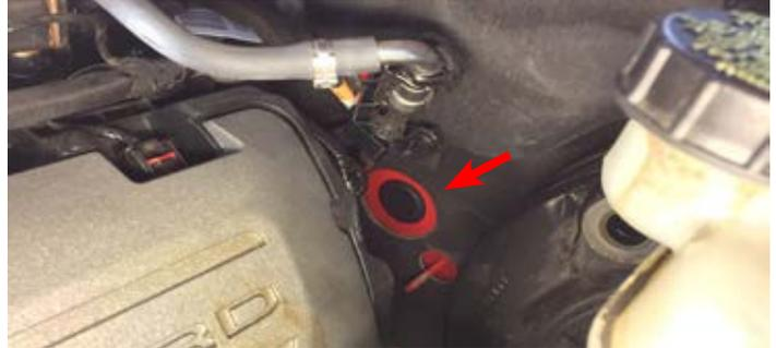
26. Remove the passenger side PCV hose from the valve cover and the intake manifold.
