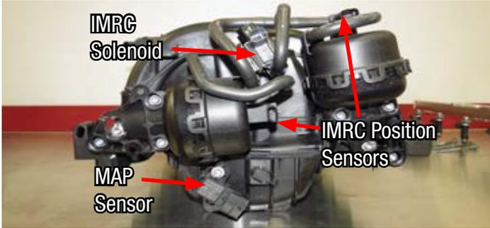
36. Make sure the IMRC harness is completely disconnected from above locations and remove the manifold. Clean the cylinder head flanges as needed and tape up the ports to prevent debris from falling into the ports. **NOTE:** Adjust the upper radiator hose clamp position to point more towards the driver's side of the vehicle. The supercharger housing will be occupying this space later. (See arrow)
