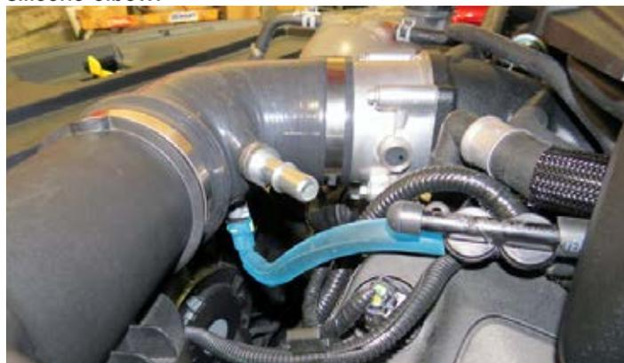
109. Connect the 90° fitting on the supplied driver side PCV hose to the driver side valve cover. Connect the other end to the fitting on the silicone elbow.
