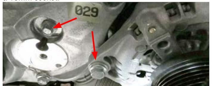
46. Secure the idler bracket by installing bolts from Bag # 2. The M10 x 110mm bolt through the ear of the alternator, the M8 x 90mm bolt into the top front cover hole, and the M10 x 45mm bolt through the lower hole that was used to secure the stock tensioner. Use blue thread lock fluid on all of the bolt threads and torque all bolts to 22 ft-lbs.
