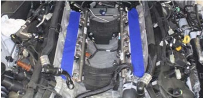
37. Remove the IMRC Solenoid from the manifold. Reconnect to the harness and zip tie out of the way. The solenoid will not be used but **MUST** be plugged in for proper engine operation.
