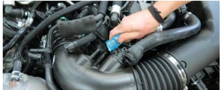
19. Remove the additional brake aspirator hose from the air inlet tube.
