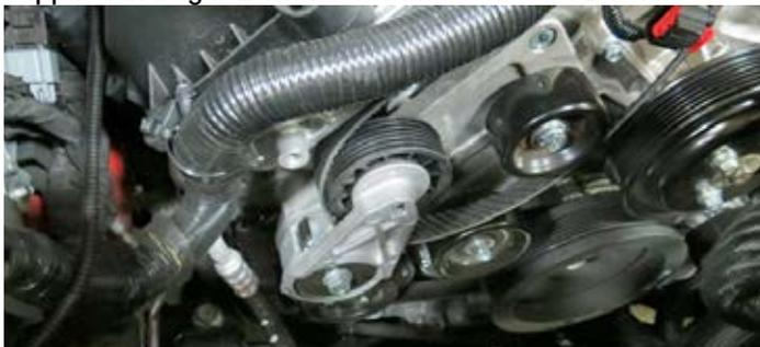
49. Using the M8 x 20mm bolts and M8 washers supplied in Bag # 2, install two idler pulleys to the tensioner bracket. The top idler pulley is 65mm and the lower idler is 76mm. Add a small amount of blue thread lock fluid to the threads ONLY, do not allow excess thread lock fluid to drip onto the pulley's bearings. Torque the bolts to 18 ft-lbs.
