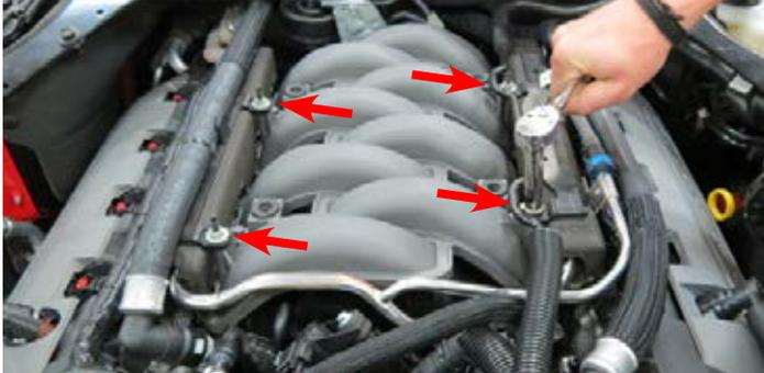
29. Remove the retaining brackets and the foam insulators from the fuel rails.
