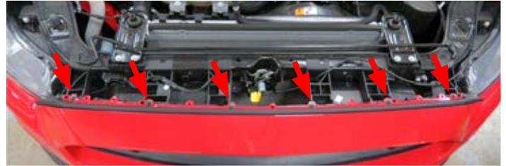
5. Using a 5.5mm socket, remove two (2) bolts under the weather stripping, one per side.
