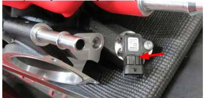
39. Install the TMAP on the driver's side of the manifold. Plug the harness into both the TMAP and MAP sensors. NOTE: Driver's side TMAP lead may need to be extended.
