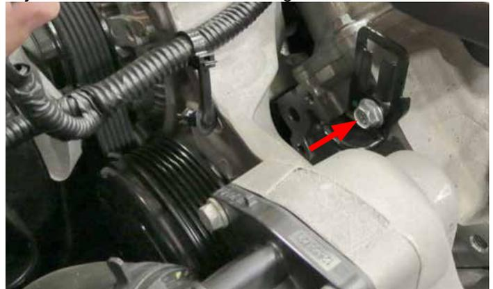
32. Reconnect the actuator solenoid connector and reattach the solenoid to the solenoid bracket.
