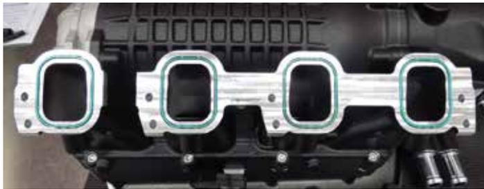
27. Remove the protective tape from the cylinder head ports. With help from an assistant, carefully lower the supercharger onto the car.
