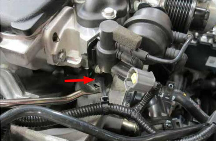
10. Disconnect the EVAP solenoid connector.
