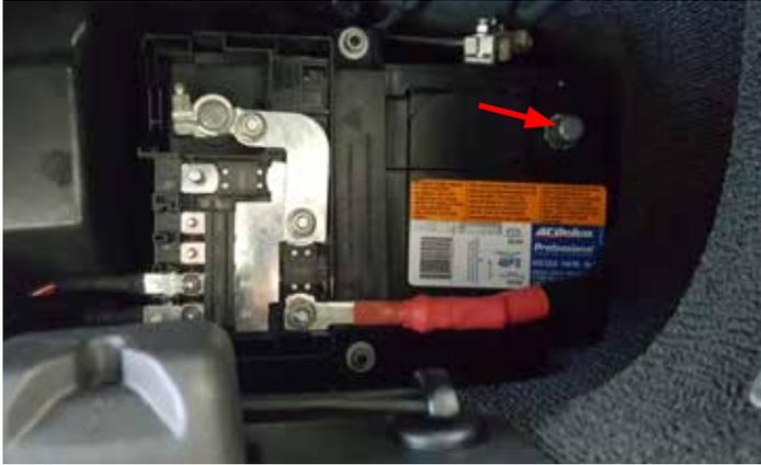
**2. CAMARO:** Open the trunk and access the battery via the door on the passenger side trunk liner. Using a 10mm socket, disconnect the negative battery terminal.
