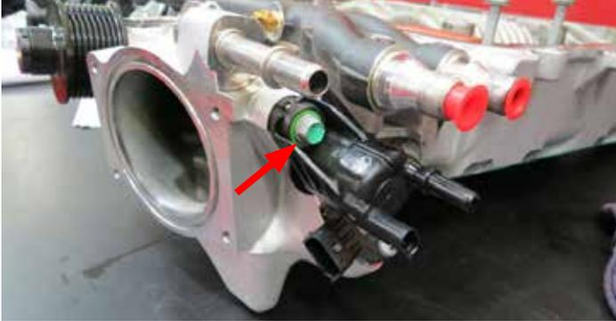
34. Using a 10mm socket, remove four (4) bolts securing the throttle body to the factory supercharger.
