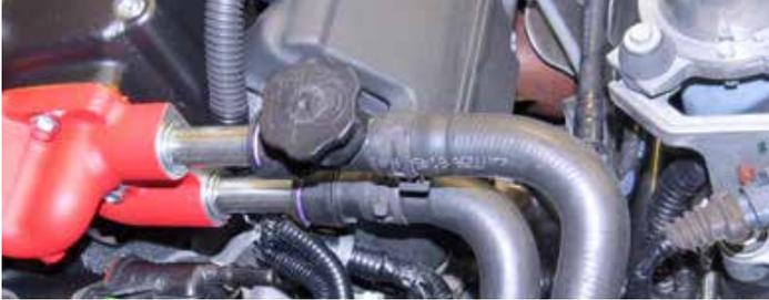
47. **CAMARO ONLY:** Install the driver and passenger side coil covers over the hoses using three (3) M6 x 40mm bolts and one (1) M6 x 35mm bolt from hardware bag 4. Oil fill cap will need to be removed before placing the driver side cover.
