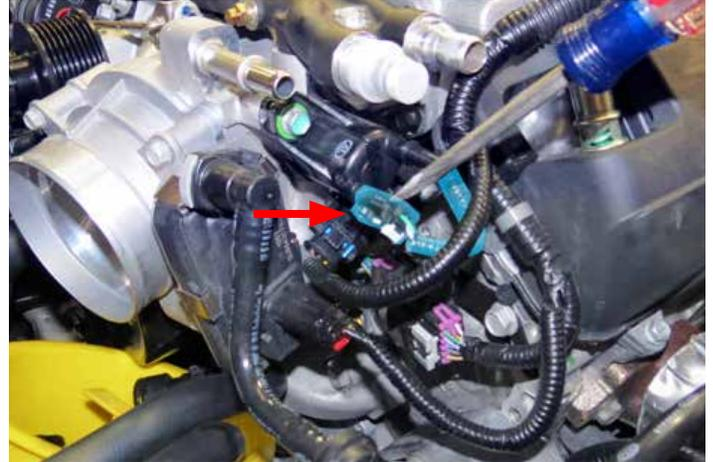
11. Disconnect the connector from the MAP sensor located under the EVAP solenoid.
