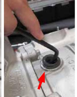
**23.** Using a hammer and a socket that is roughly the same diameter as the PCV seal, gently tap in the seal into the supercharger until the seal is flush with the housing.
