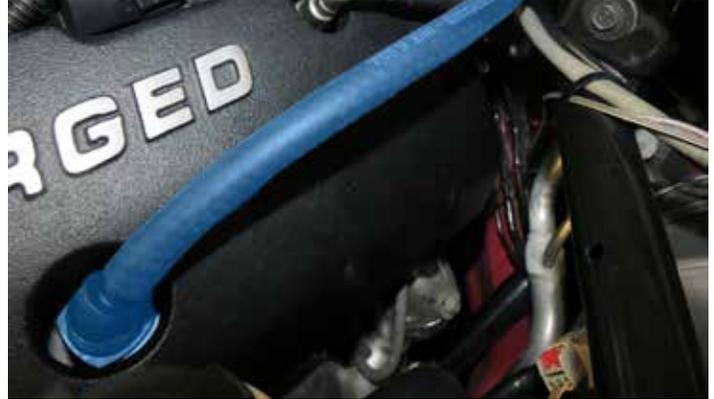
51. Install the supplied bypass hose onto the fitting on the bottom of the actuator then over the cover to the manifold as shown.
