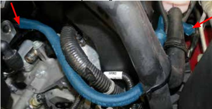
42. Using a breaker bar, rotate the tensioner counterclockwise and install the supercharger belt using the routing diagram below.
