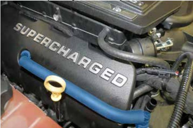
50. Connect driver side pcv hose through the hole in the coil cover.
