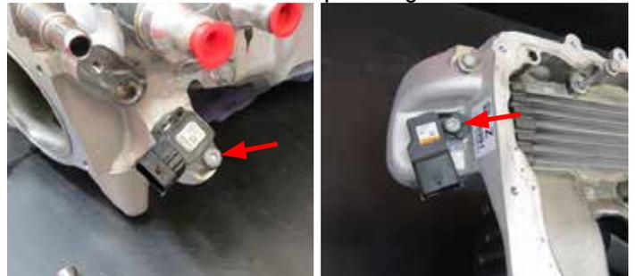
38. Using a Torx T30 screwdriver, install the MAP sensor to the supercharger nose using the factory bolt.
