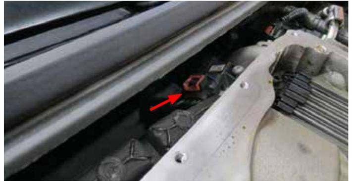
17. With the help from an assistant, carefully remove the supercharger manifold and set aside.
