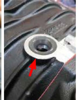
**24.** Remove the factory O-ring gaskets from the intake manifold.
