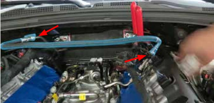
**20.** Check for clearance on the foam insulator. This may need trimming to clear the larger supercharger housing.
