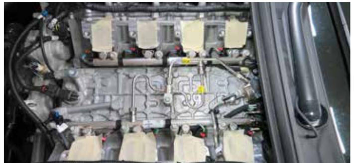
**19. CAMARO ONLY:** Remove the retaining clip on the fuel feed line. Using a 3/8" fuel line tool, disconnect the fuel line from the fuel line extension and from the factory hardline. Install the supplied fuel line as shown. **CAUTION: Place a shop rag around the fuel line to prevent fuel from spraying.**
