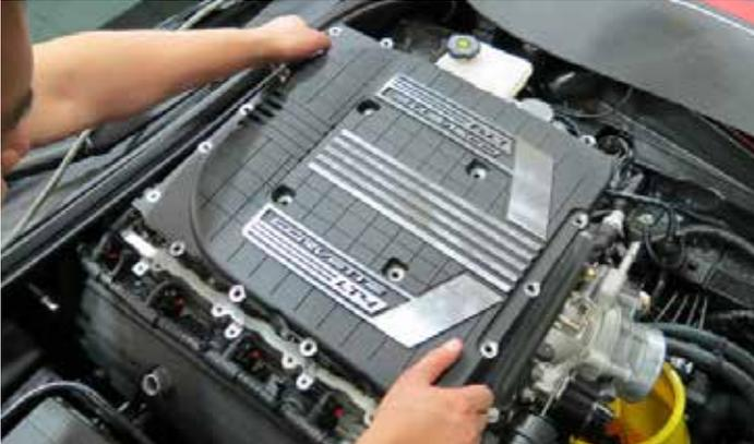
15. Using a 10mm socket, remove ten (10) bolts securing the supercharger manifold to the cylinder heads.
