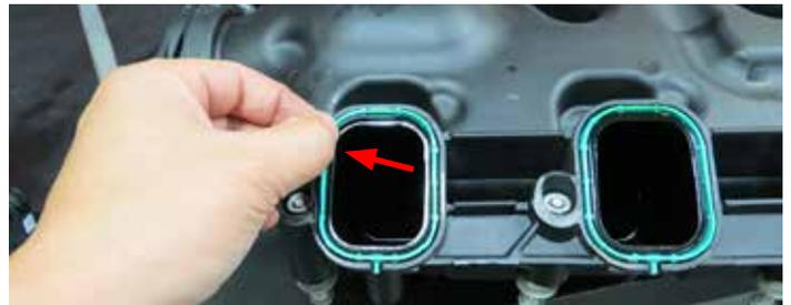
25. Clean and inspect the O-ring gaskets. Replace torn or damage O-rings as needed. Using a razor blade remove the tips off all eight (8) factory O-ring gaskets.
