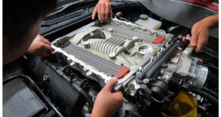
18. Cover the ports with protective tape to keep out debris. Remove the black foam insulator from the valley and set aside.
