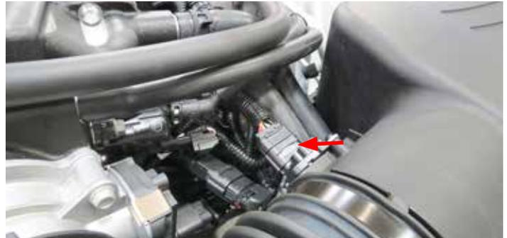
44. Using the supplied worm clamps, secure the inlet elbow to the throttle body and the air intake box.
