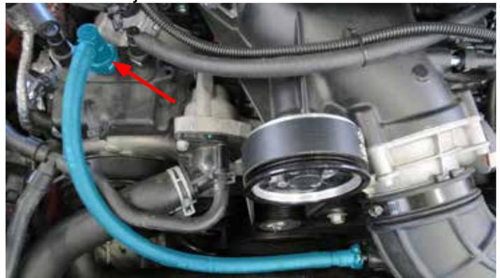
46. Connect the factory coolant hoses to the fittings on the water crossover.
