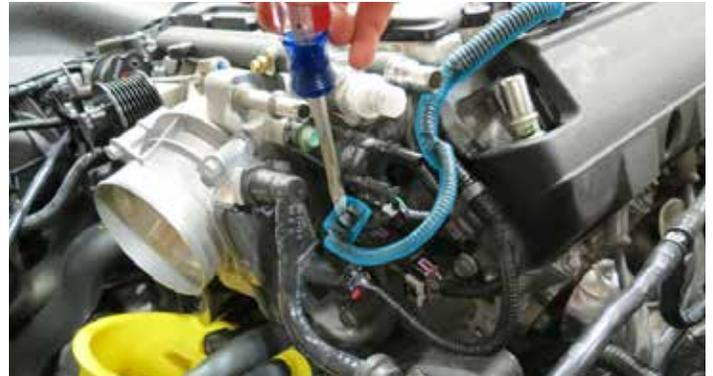
12. Release the blue locking clip on the electronic throttle body connector and remove the connector from the throttle body.
