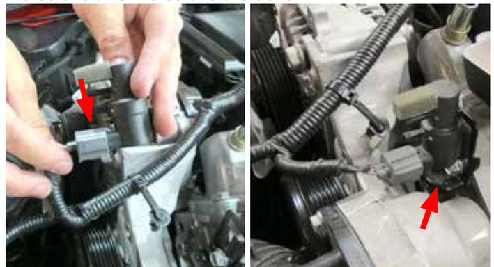
33. Using a 10mm socket, remove the EVAP solenoid from the factory supercharger.
