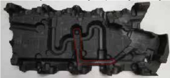
**21.** Reinstall the foam valley insulator onto the valley making sure it is seated properly.
