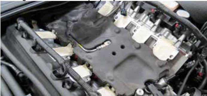
**22.** Using a pry tool with smooth edges, remove the factory PCV seal from the bottom of the factory supercharger. **TIP:** It's best to pry the seal on the metal base as to not tear the upper rubber portion. **NOTE:** In the event this PCV Seal is missing or damaged contact Edelbrock Tech Support @ 800-416-8628 to purchase a replacement seal P/N 51-4301.
