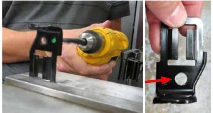
31. Using the M8 x 30mm bolt and the 3/8" CAD washer from the hardware bag, secure the actuator bracket to the front of the passenger side cylinder head. Location is adjacent to the thermostat housing.
