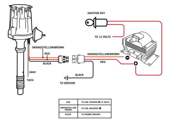
**WARNING:** This distributor is not compatible with stock points distributor coil, must use high output coil. Must bypass ballast resistor if applicable.
