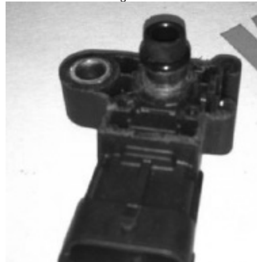
Figure 2 Re-install O'ring and install MAP sensor. Lubricate lightly with engine oil. Plug in MAP sensor using jumper provided with Engine control System kit. See Figure 3.
