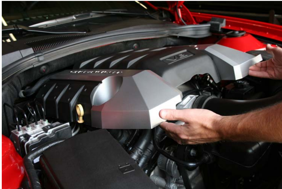
Step 2: Remove intake cover
