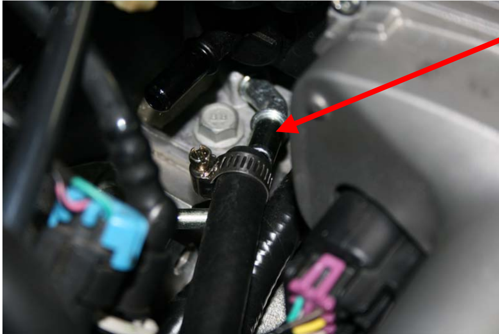
Step 16: Push hose over nipple on manifold behind throttle body, and tighten clamp
