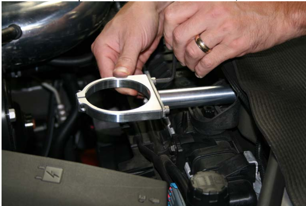
Step 14: Install and tighten billet clamp to stainless bracket using (2) 1/4 x 5/8" socket head cap screws
