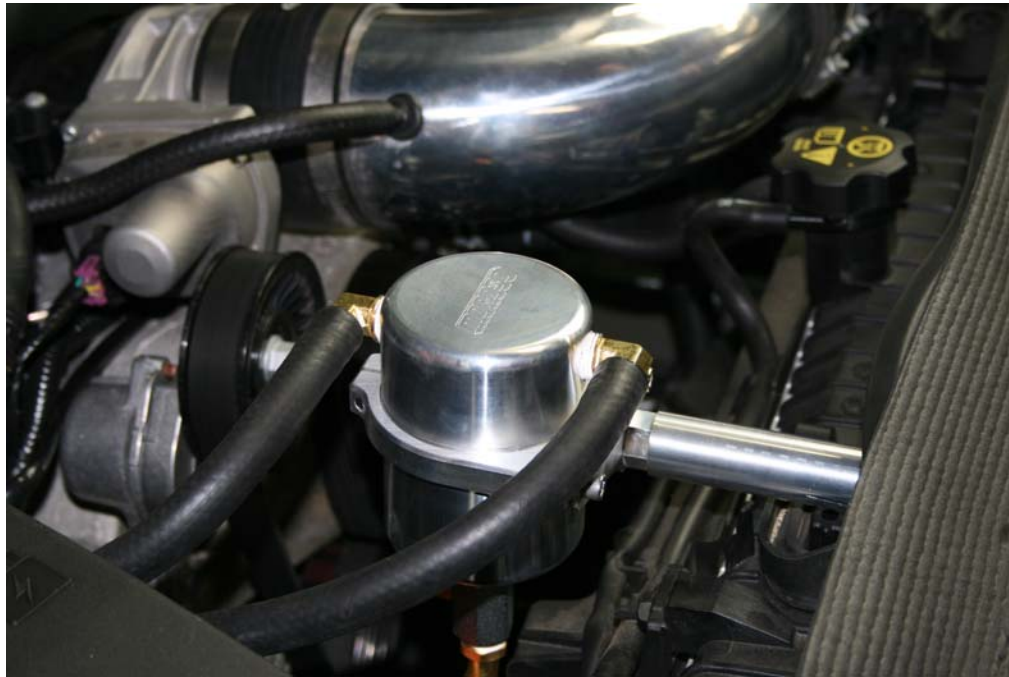
Step 26: Push hose over barbed fitting
