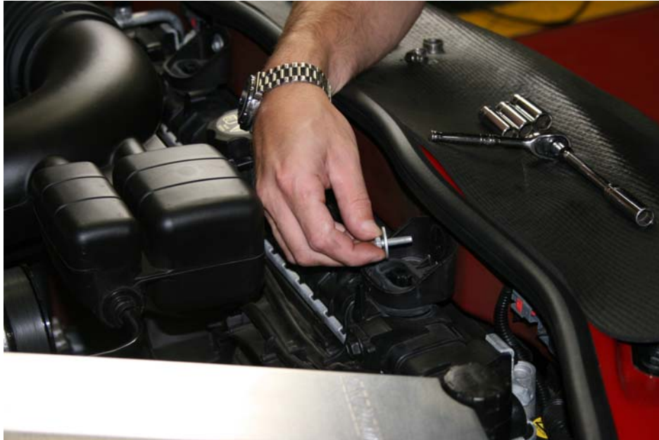
Step 8: Locate radiator, mounting bolt on passenger side and remove
