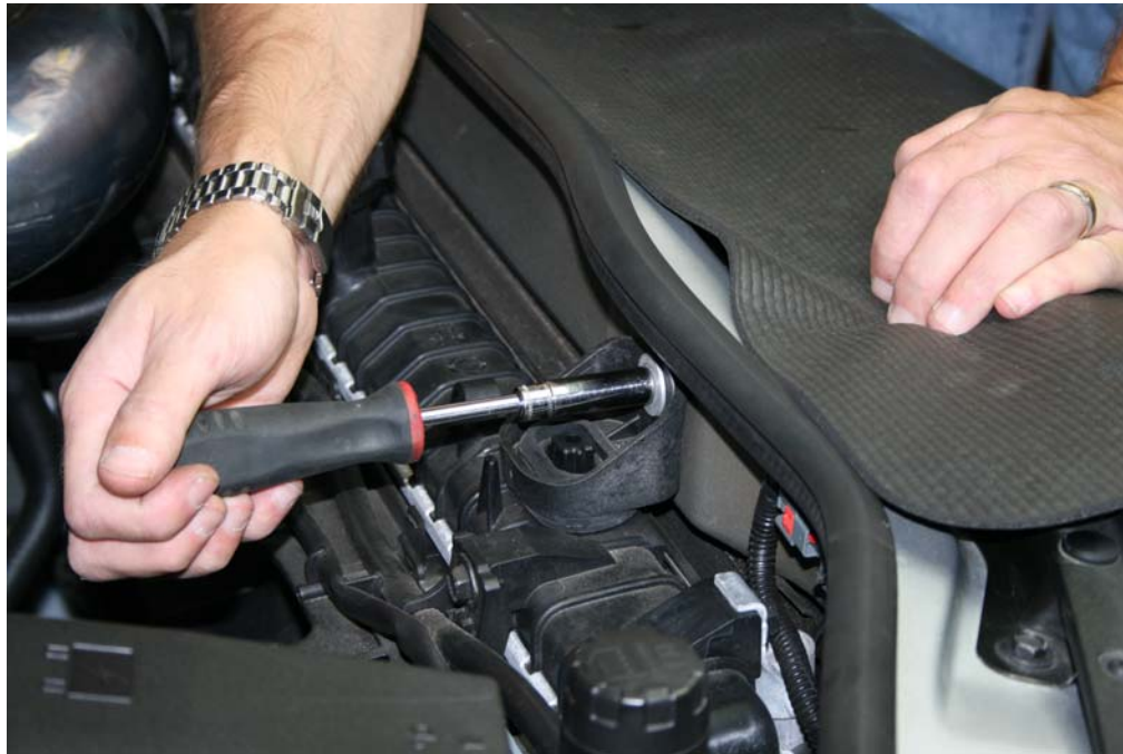
Step 9: Locate radiator, mounting bolt on passenger side and remove
