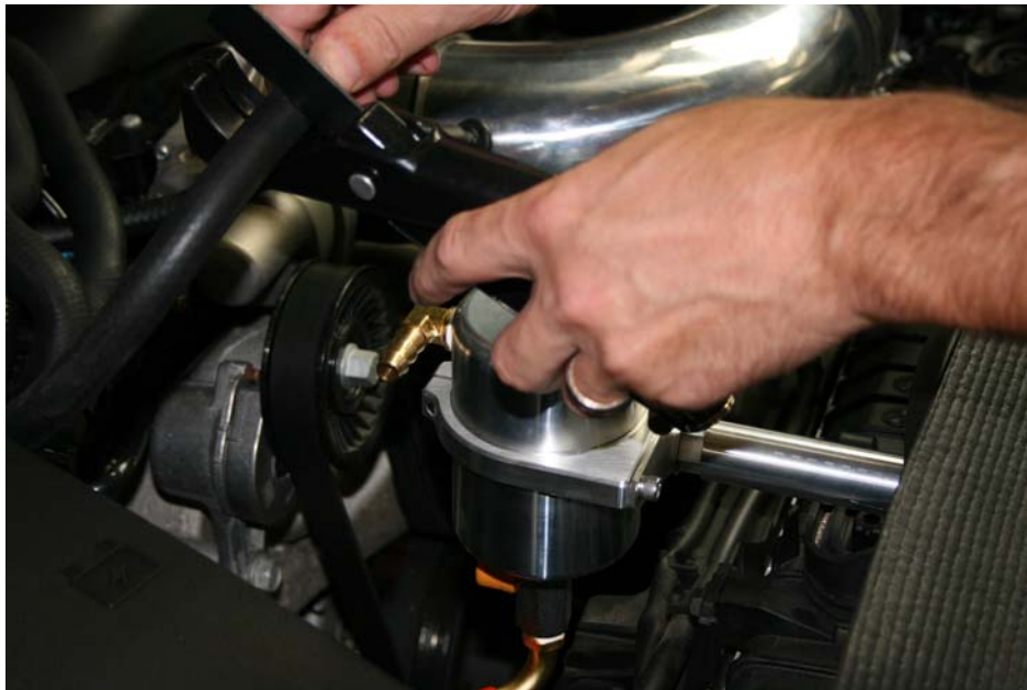
Step 18: Mark and trim hose to length if necessary
