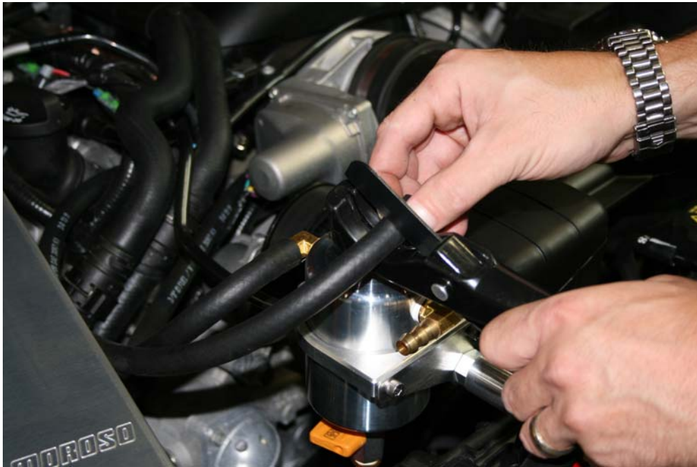
Step 23: Trim hose as necessary
