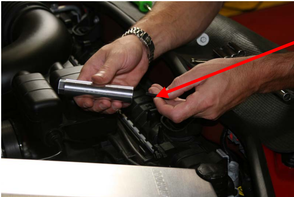
Step 9: Install and tighten 6mm stud into billet mount as shown (note billet mount contains metric and standard threads, thread stud into round end of mount)
