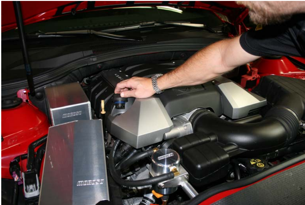
Step 27: Reinstall oil fill cap
