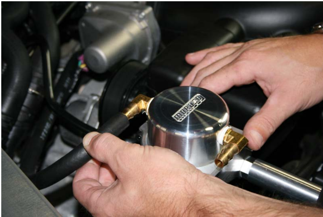
Step 18: Trim hose as necessary
