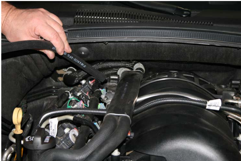
Step 20: Route one end of 5 ft hose under heater hoses and behind intake manifold
