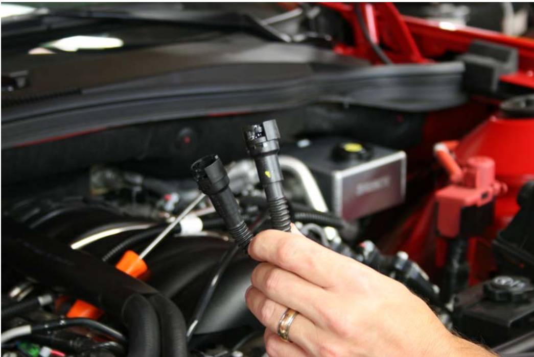
Step 7: Remove PCV line from vehicle
