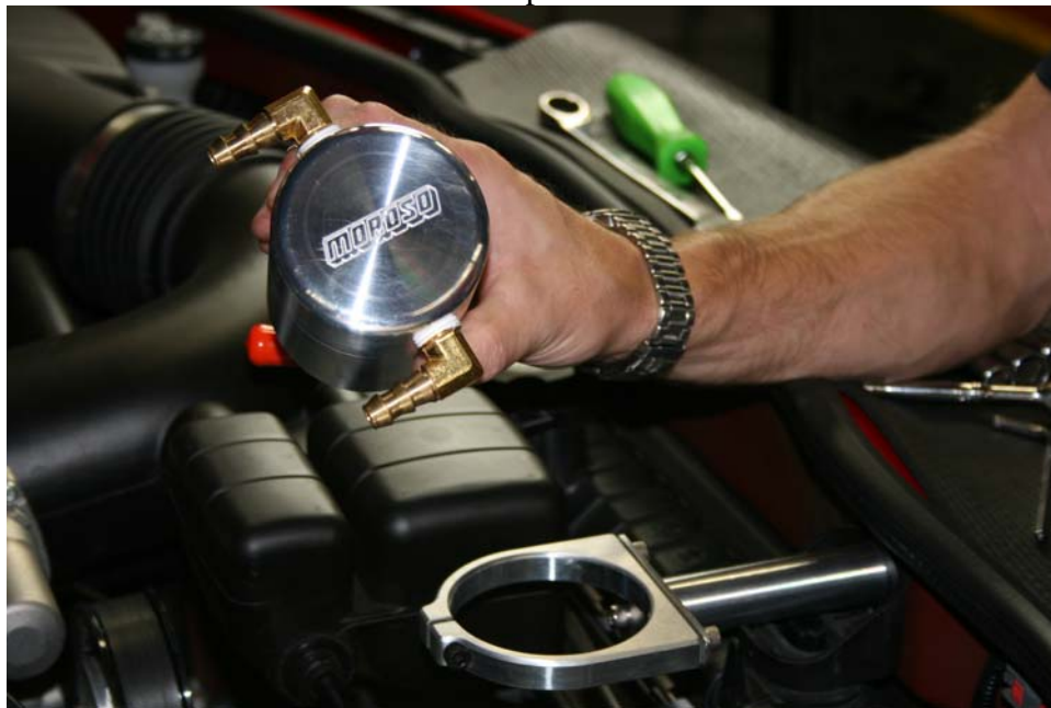
Step 13: Assemble air oil separator as shown, apply Teflon tape to all fittings
