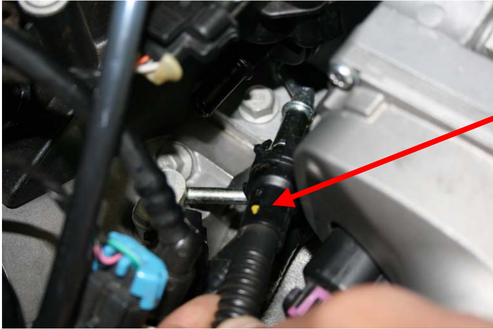
Step 6: Remove other end of PCV line
