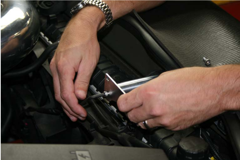
Step 13: Install and tighten stainless bracket to billet mount using 1/4x5/8" socket head cap screw (Blue LOCTITE recommended)
