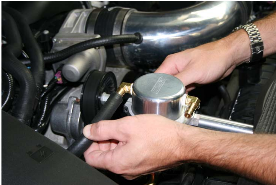
Step 19: Push hose over barbed fitting
