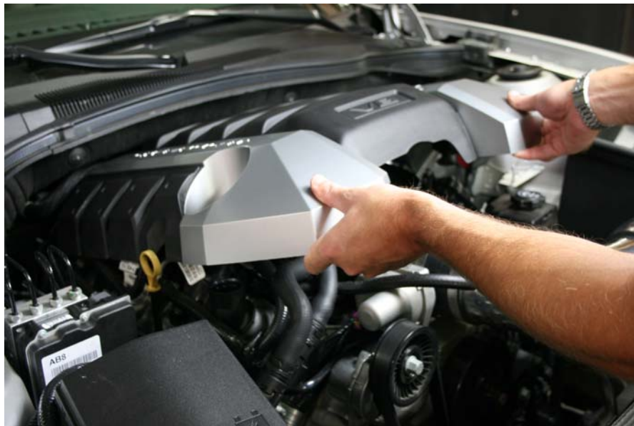
Step 2: Remove intake cover
