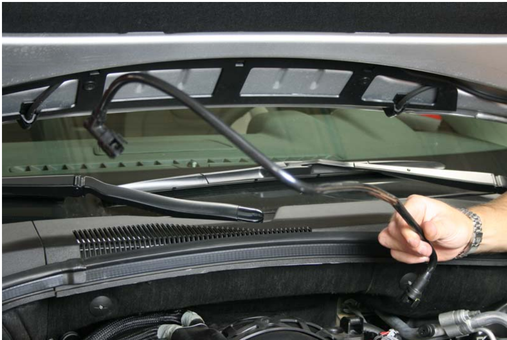
Step 8: Remove PCV line from vehicle
