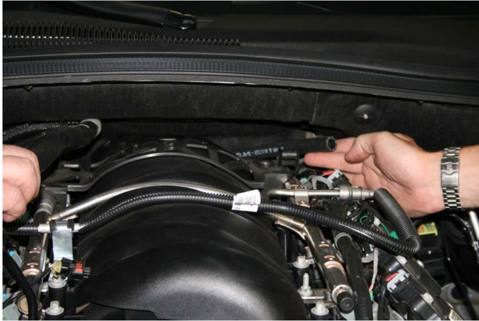
Step 21: Continue routing hose behind intake manifold to valve cover nipple
