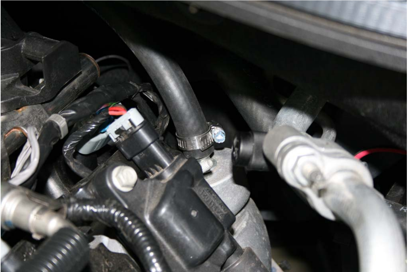
Step 23: Push hose over nipple and tighten clamp
