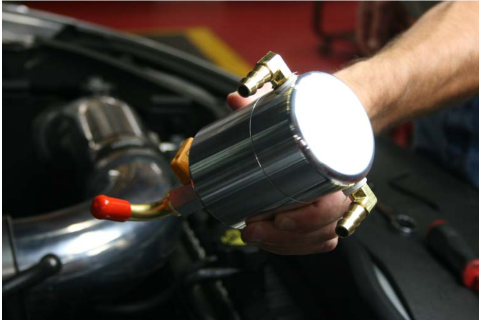
Step 10: Assemble air oil separator as shown, apply Teflon tape to all fittings
