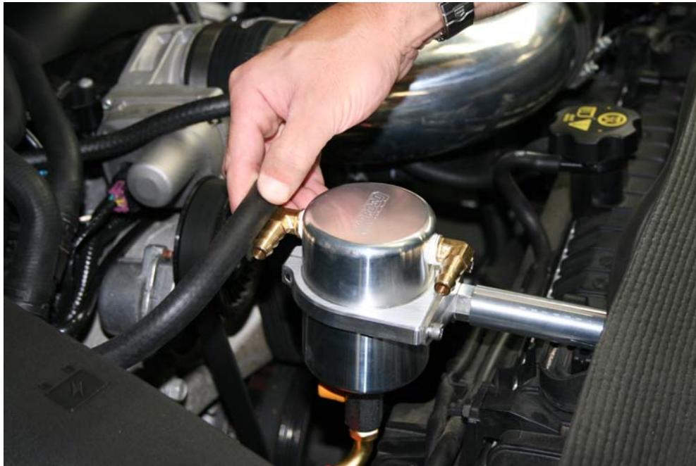
Step 17: Route other end of hose to Air Oil Separator as shown
