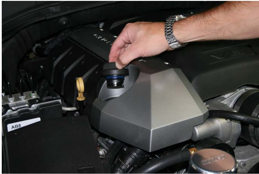
Step 29: Reinstall oil fill cap
