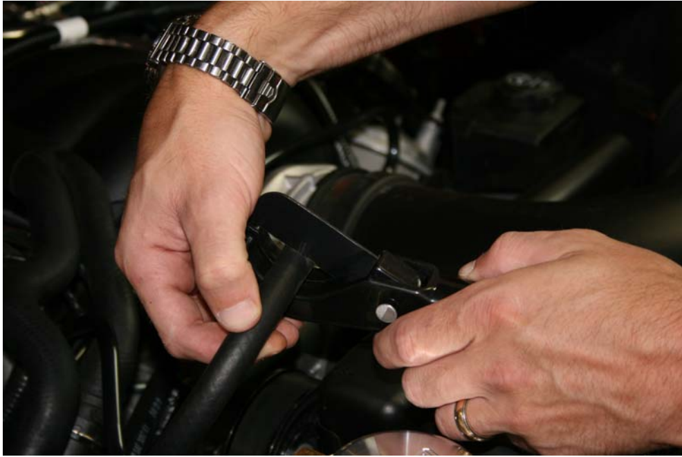
Step 18: Trim hose as necessary
