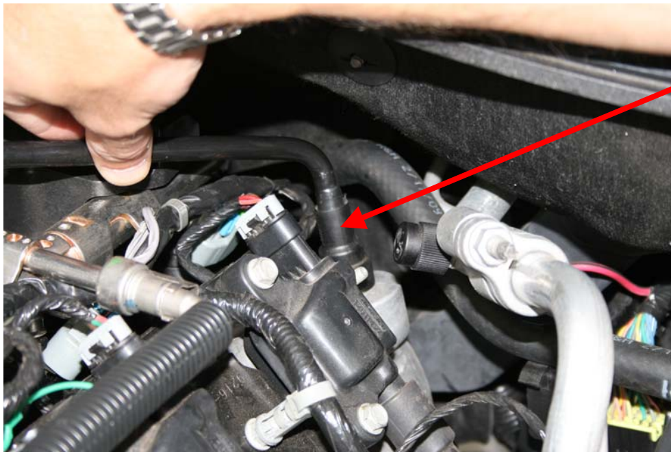
Step 6: Locate other end of PCV line, on rear of drivers side valve cover
