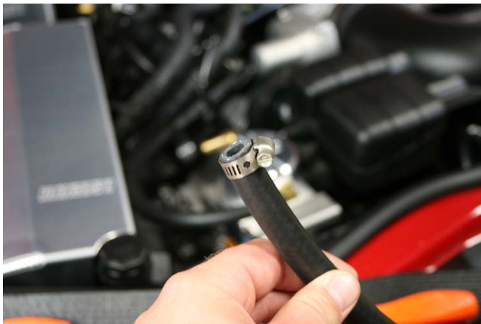
Step 20: Place hose clamp over one end of 5ft long hose
