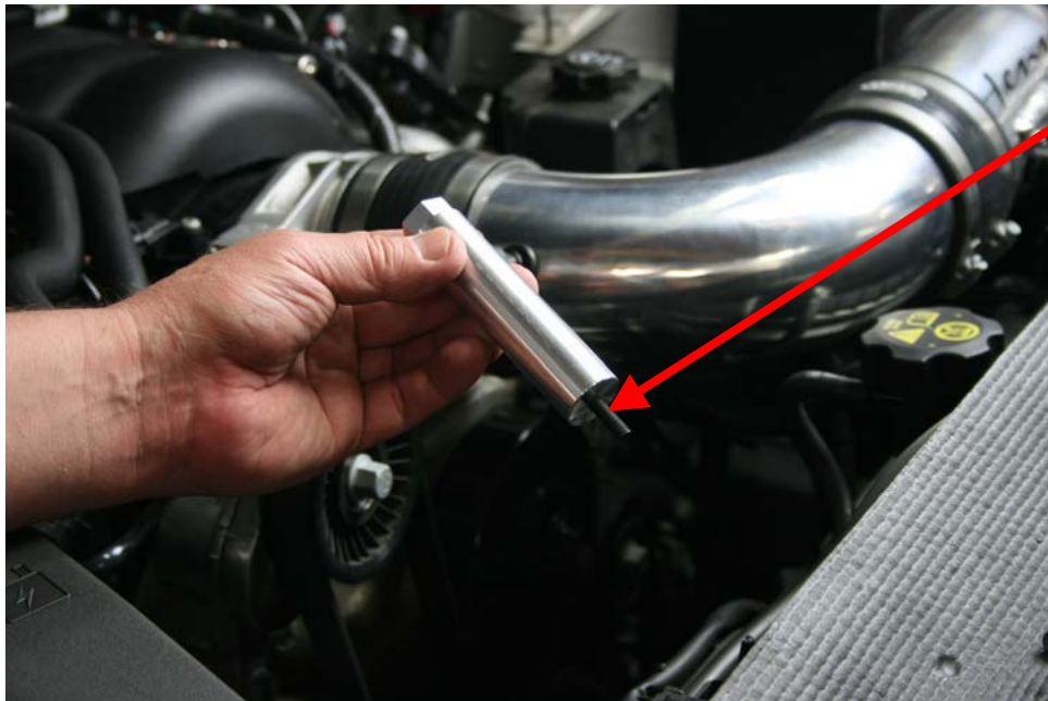
Step 11: Install and tighten 6mm stud into billet mount as shown (note billet mount contains metric and standard threads, thread stud into round end of mount)
