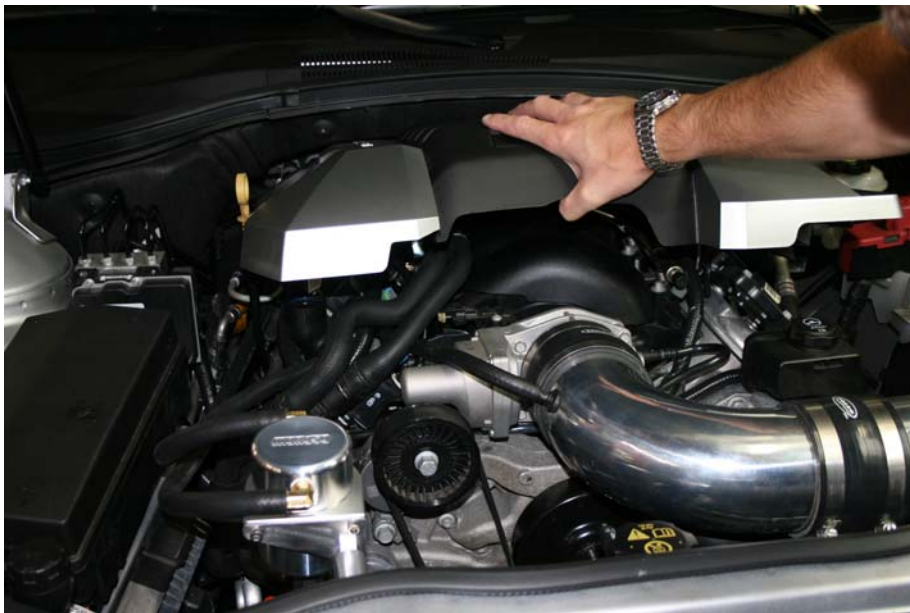
Step 28: Reinstall intake cover
