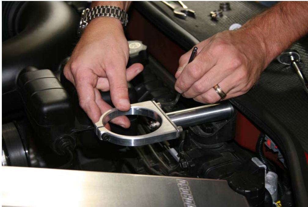
Step 12: Install and tighten billet clamp to stainless bracket using (2) 1/4 x5/8" socket head cap screws
