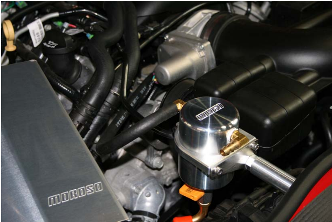
Step 19: Push hose over barbed fitting
