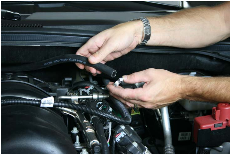
Step 22: Place hose clamp over hose
