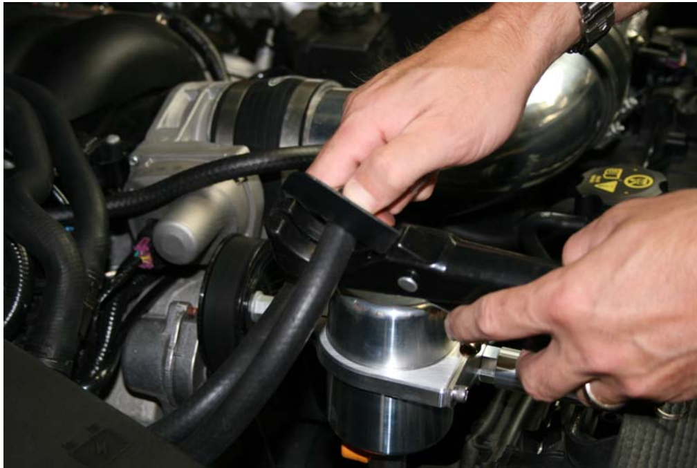
Step 25: Mark and trim hose as necessary
