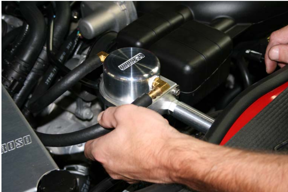
Step 24: Push hose over barbed fitting
