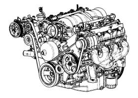
Not included is a required six-rib belt, length such that the tensioner indicator arrow is between the max and min marks. See the following table for suggested belt lengths and Gates/Delco part numbers.
