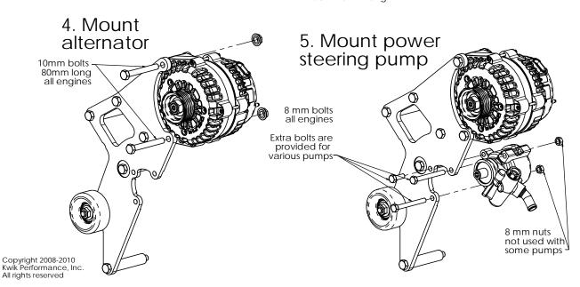
6. Torque fasteners: 12mm: 50 ft-lbs 10mm: 37 ft-lbs 8mm: 15 ft-lbs
