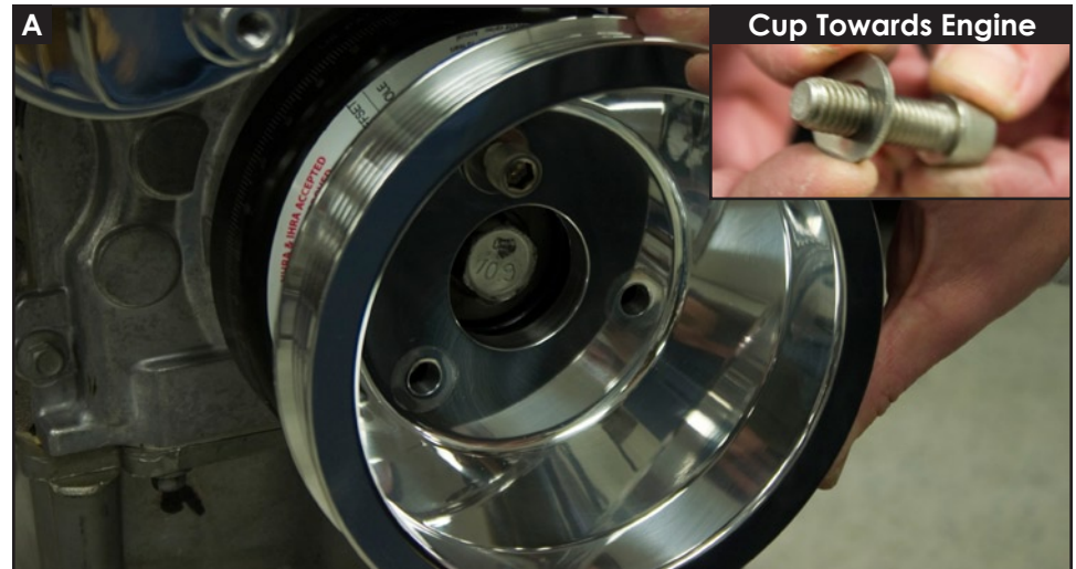
Figure 7: Install Crankshaft Pulley
