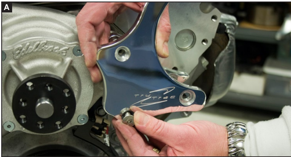
Figure 5: Install Alternator Bridge Bracket
