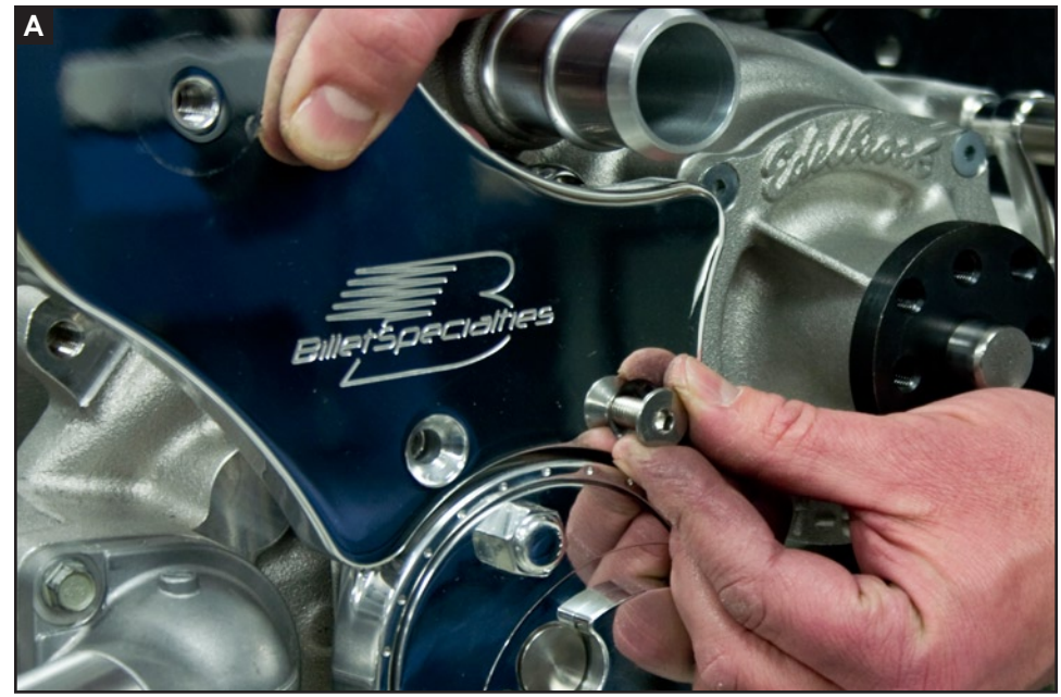
Figure 4: Install Idler Bridge Bracket
