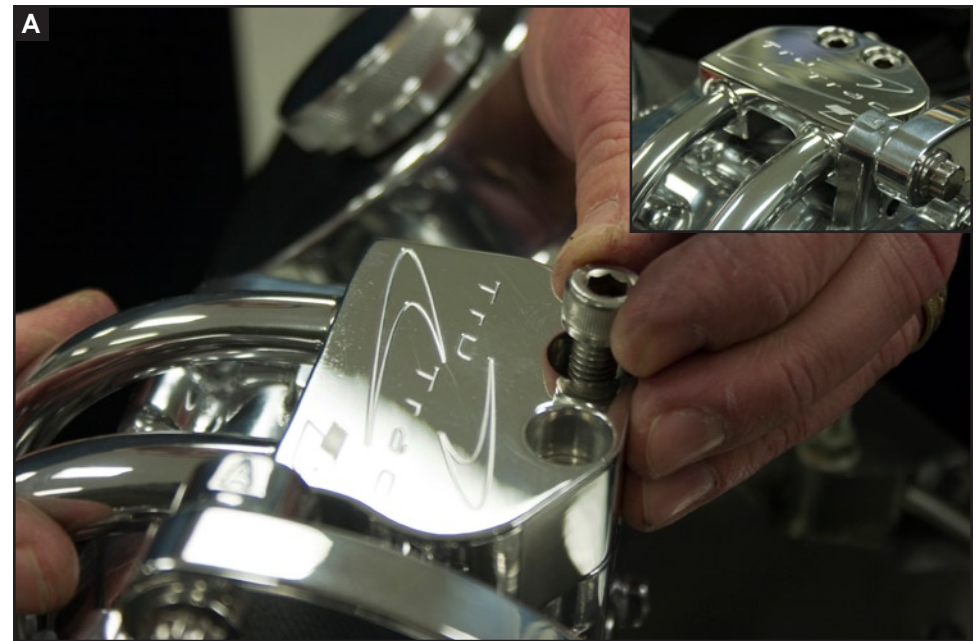
Figure 14: Install Compressor Manifold
