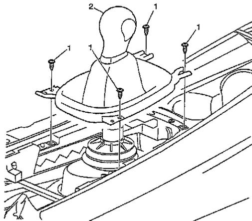
Next remove the 4 fasteners that hold the shifter assembly to the floor using a 10mm socket.
