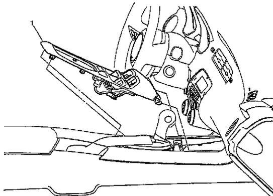
Remove the transmission control lever knob and boot assembly as shown below.
