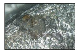
**Ethanol Corrosion Can Quickly Destroy Your Carburetor!**
