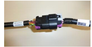
Bulkhead Connection
